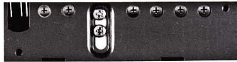
Servo adjustment trimmers are located under the splicing block for easy access and fast maintenance.
